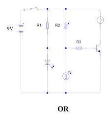
(d) When the circuit was built it was found not to be very sensitive. Redraw the circuit indicating two changes you could make so that it is more sensitive to changing light levels.
